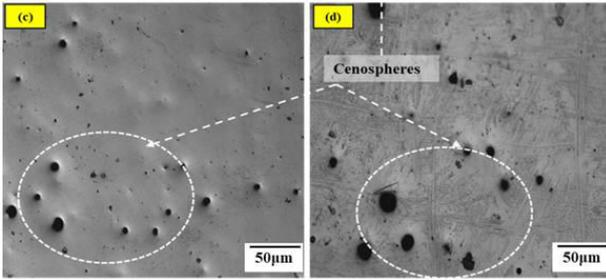
Fig 6. Microstructure Characterization of Al3003- Cenospheres MMC's using Optical Microscope.
