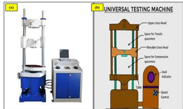
Fig 5. (a) Universal Testing Machine (b) UTM Line Diagram
