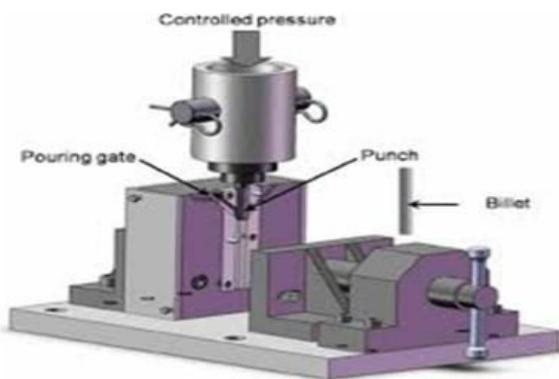
1. Squeeze casting setup Fig
