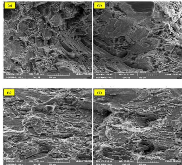
Fig 9. Tensile surface Fractographs of Al3003-Cenospheres MMC's
