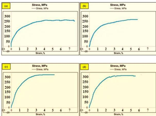
Fig 7. Stress Strain curve of Al3003/Cenosphere MMC's
