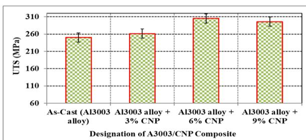
Fig 8. Tensile test values (UTS) of Al3003-Cenospheres MMC's
