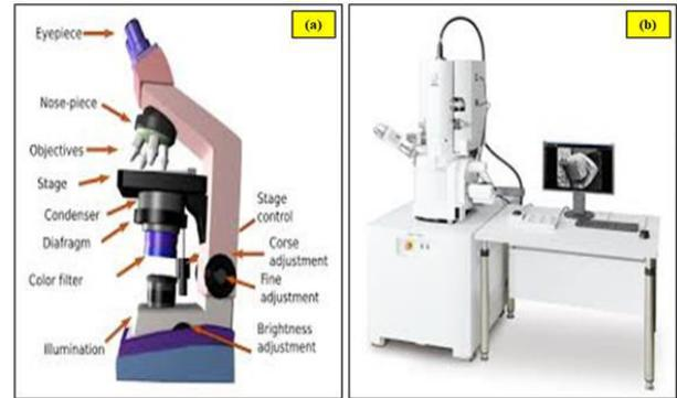
Fig 4. (a) Optical Microscope (b) Scanning Electron Microscope
